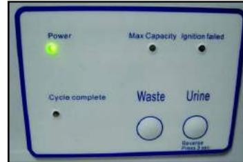
A control board monitors the amount of usages and its burn process. Indication lights come onto a display panel if there is an error or if the process has finished its burn cycles. The panel also has the two flush buttons that one has to push in order to start the burn cycle.
